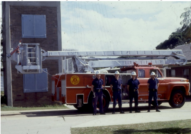
Above: Redcliffe firemen stand proudly beside their new HP. With only two stabiliser arms at the rear the F750 was a little unstable.
