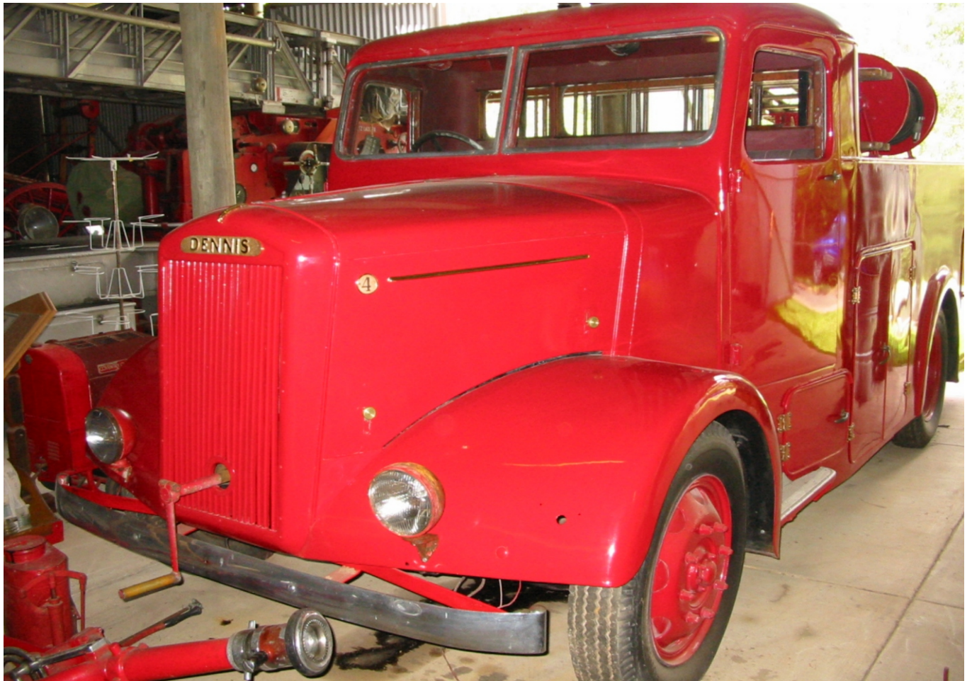
Above: 1947 Dennis F1, ex NSWFB car 19, currently undergoing restoration at the Museum. Fitted with a 400 GPM pump.
