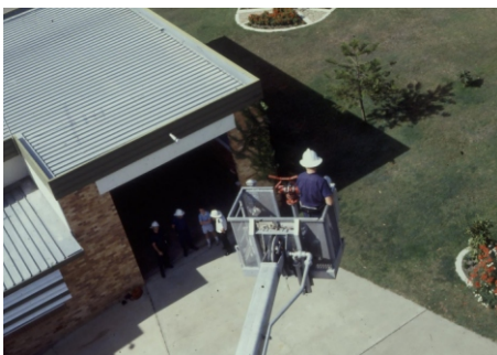
Above: Redcliffe firemen stand proudly beside their new HP. With only two stabiliser arms at the rear the F750 was a little unstable.
