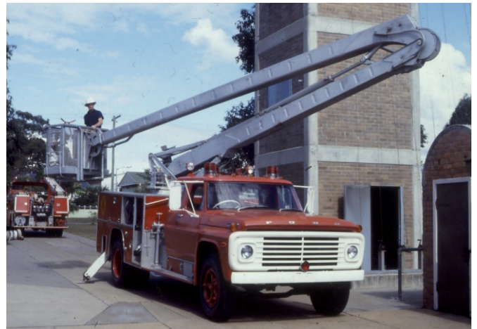
Above: Redcliffe firemen stand proudly beside their new HP. With only two stabiliser arms at the rear the F750 was a little unstable.
